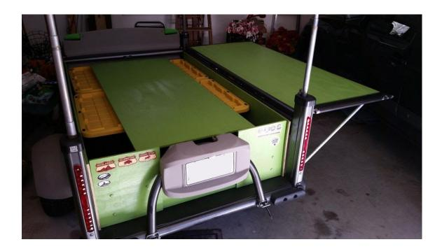
14) I used 2 or 3 furniture felt stick-on dots along the side rails, these keep the top edge of the cargo sideboards from smacking against the rails while bouncing down the road.
