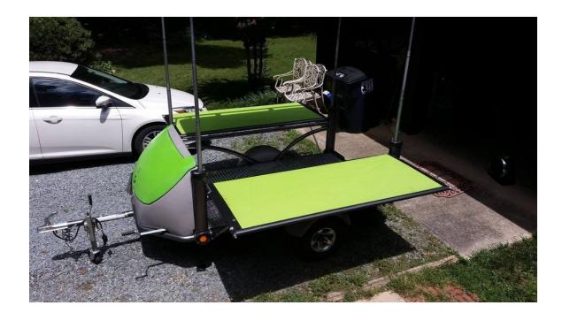
3) I'm no carpenter. I improvised this for my rear panel. The two plywood ends were left-over from the store cuts. The only extra piece of wood (other than the two plywood sheets) is the board that runs between these two pieces.
