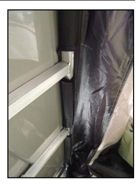
*Step 16:* At the bottom of the front wall loop the small Velcro straps around the bottom cross bar and secure loosely as shown.
