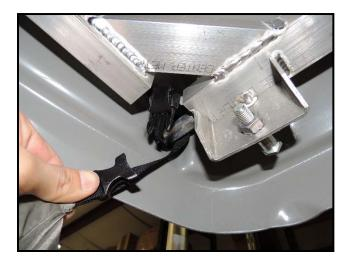
*Step 9:* Snap together the male and female ends of the connector.
