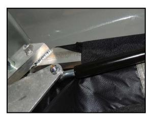
*Step 14:* Proceed to loop and attach the Velcro flats around the remainder of the top frame.
